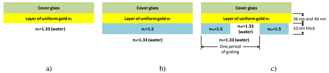
Figure 5.1 shows samples used in this study a) bare gold case b) coated gold case and c) grating case
