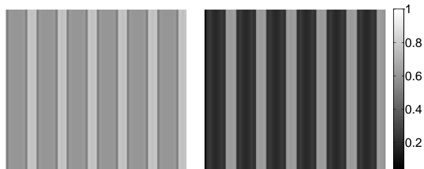
Figure 4.22 shows linescan images of a) 30 nm of gold and b) 50 nm of gold when the mask width was 5 degrees taken at 47.5 degrees centre of mask position r polarisation
