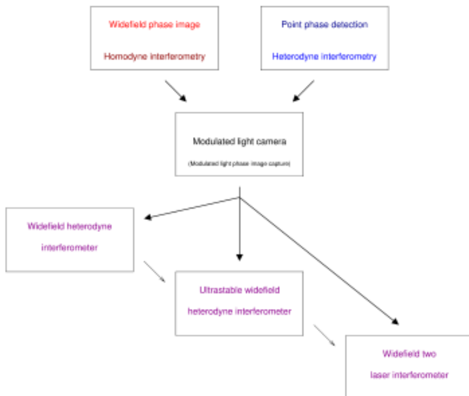
Figure 1.12: A flow diagram showing the ideas used in implementing the interferometer systems discussed. The camera is used to capture widefield heterodyne interferograms. Modifying the setup produces an ultrastable configuration, which can be used to capture two laser interferograms.
