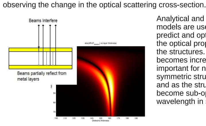
Analytical and FE models are used to predict and optimise the optical properties of the structures. FE becomes increasingly important for non symmetric structures and as the structures become sub-optical wavelength in size.
